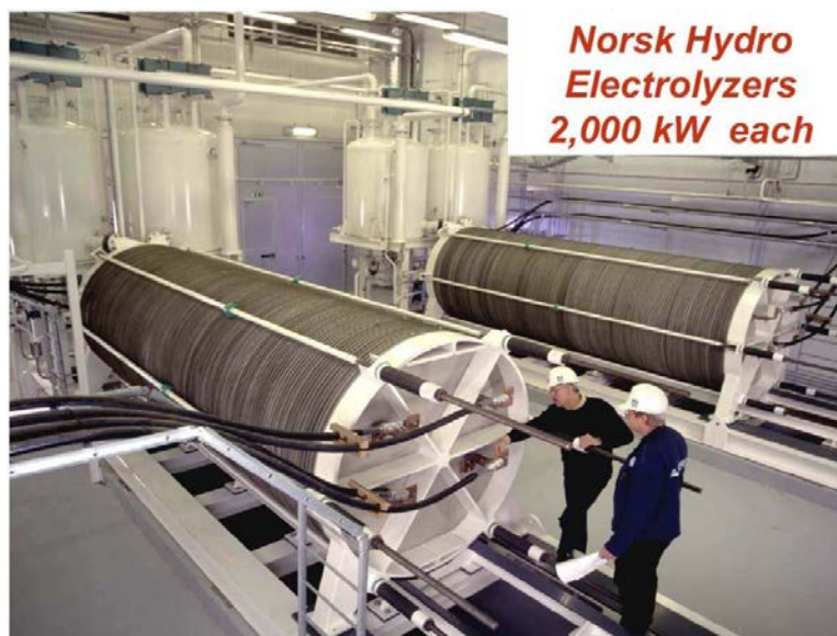
Figure 3.6 Megawatt Scale Hydrogen Production By Electrolysis
